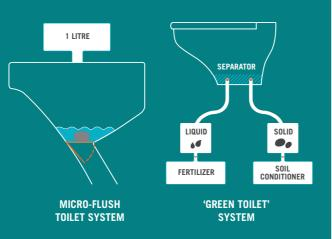
The Micro-Flush Toilet System improves the water efficiency of toilet and sewage systems.
